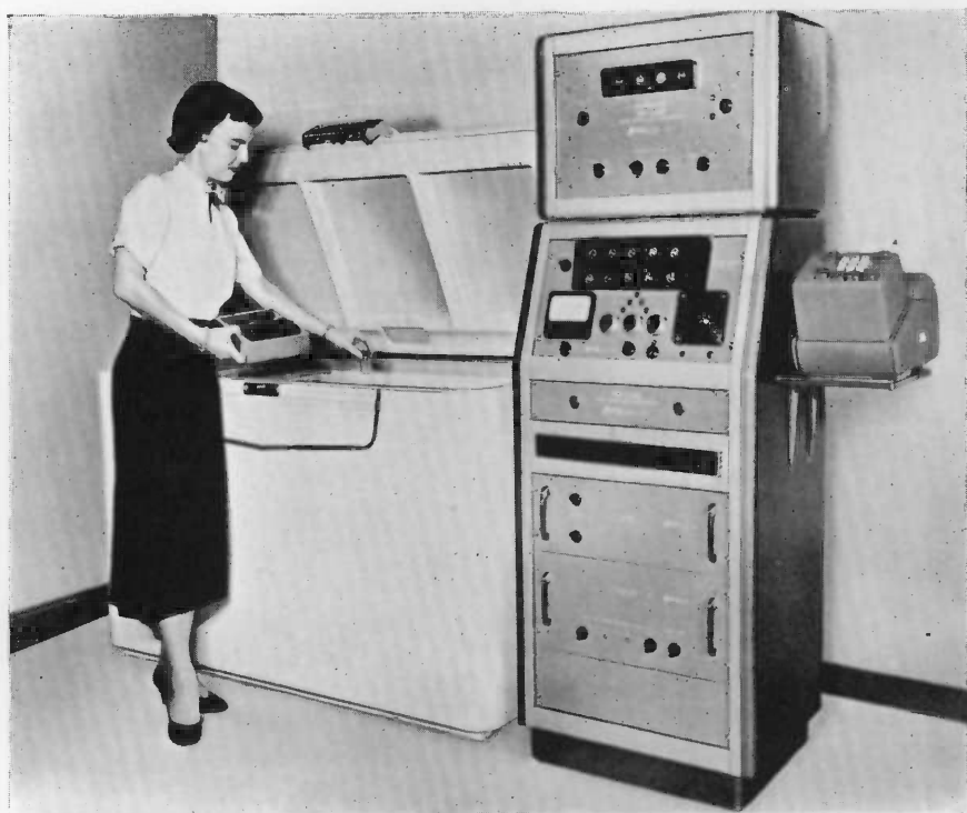
Fig. 16. Overall view of the automatic Tri-Carb liquid scintillation spectrometer showing samples being loaded into the turntable inside the freezer prior to automatic counting.
