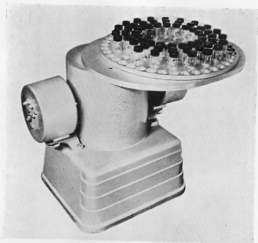
Fig. 15. Iron-shielded sample chamber used for automatic counting of up to 100 samples in the automatic Tri-Carb spectrometer.
