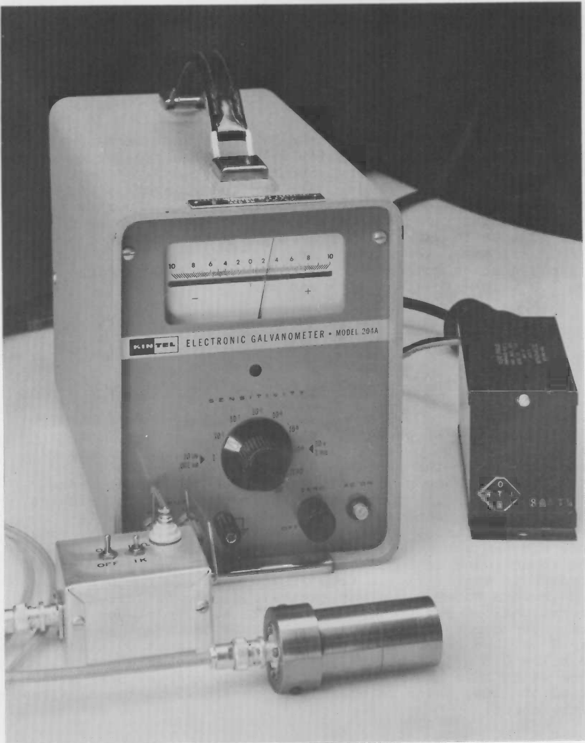
Fig. 2. Photovoltaic cell detector and galvanometer.
