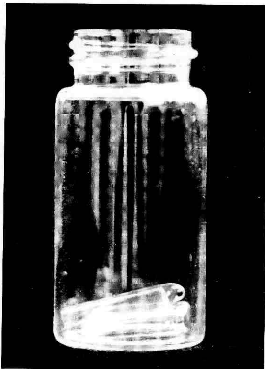
Fig.2. Scintillation vial with reaction tube (without scintillator) for direct measurements.
