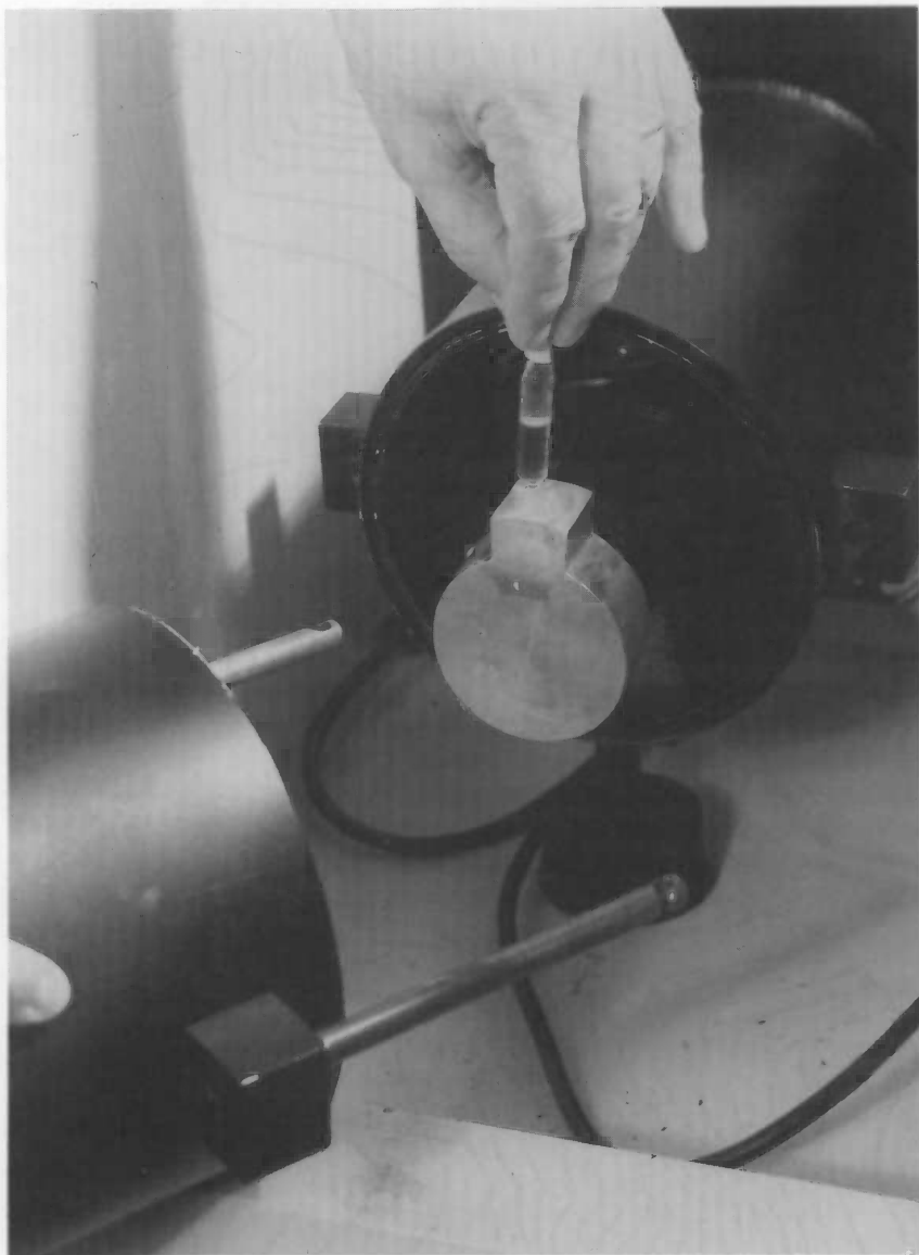
Figure 2. Experimental light-tight enclosure in which various reflector arrangements were tested.
