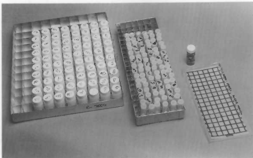
Figure 8. There is a 95% reduction in the volume of disposables when using filter mats. A 96 sample filter can be contained in a single standard vial.
