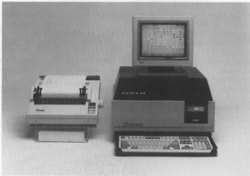
Figure 4. Packard Matrix™ 96, 96 sample direct beta counter.
