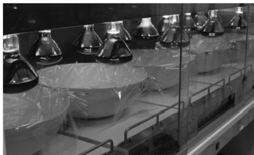
Figure 2 Concentration of lake water samples by evaporation. A thin film makes it easy to take the evaporation residue off of the crucible.
